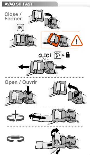
6. EN 358: 2018 harness for work positioning and restraint
