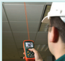
Model AN200 features built-in non-contact IR Thermometer to measure surface temperature that may be hard to reach
