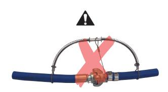
Incorrect Installation King Safety Cable is not installed in the extended position (too much slack). When a pressurized air hose becomes accidentally uncoupled, or a hose failure occurs, the quick exhaust of air causes the hose assembly to whip violently, creating a potentially dangerous situation.
